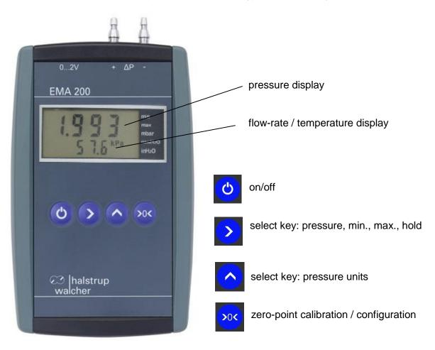
The instrument control panel consists of a keypad with four keys.
