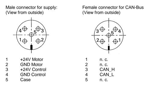
Optional it is possible to get the CAN-Bus connector-pinning according to CiA. Then the power connector is from Binder series 766 (B-coded).
