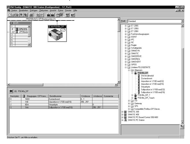
Normal operation requires only the status byte, the command byte, the target position and the actual position. Depending on the magnitude of the spindle pitch, 16 bit bytes are adequate for transferring target and actual values, thereby keeping the transfer time as short as possible.
