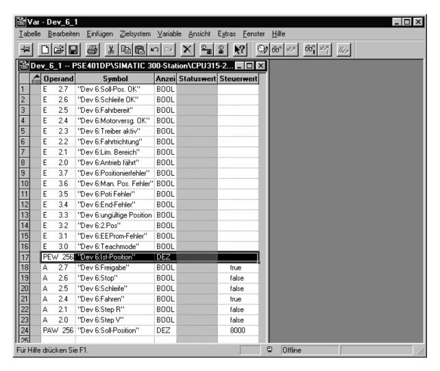
This module transfers the current actual position to the control unit in one of two different data formats. If the spindle pitch is >4.00 mm, the limited range of values restricts the positioning options. These restrictions are not an issue for the actual position module (I32).
