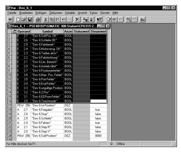
Bit 15(MSB): Target pos. OK (target position reached)
