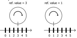
The referencing value is written either directly or by setting the actual position. 4) Setting upper mapping end:
