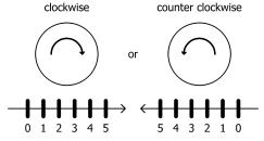
Setting numerator and denominator: The numerator and denominator determine the number of steps into which one rotation of the output shaft is divided.
