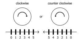
2) <u>Setting numerator and denominator</u>: The numerator and denominator determine the number of steps into which one rotation of the output shaft is divided.
