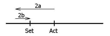
3. New setpoint position is only slightly larger than the current actual position and previously there was no positioning movement with loop (e.g. a manual movement):
