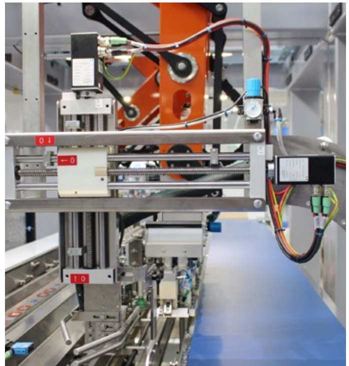
Fig. 4: Positioning systems can perform format changeovers in packaging machines quickly, precisely and at the touch of button
