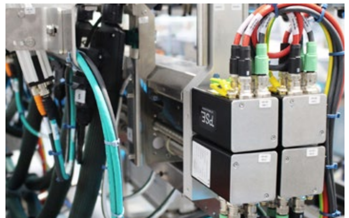
Fig. 2: Automatic adjustment of the glue application module for gluing boxes: It is vital to apply exactly the right amount of adhesive in exactly the right place.
